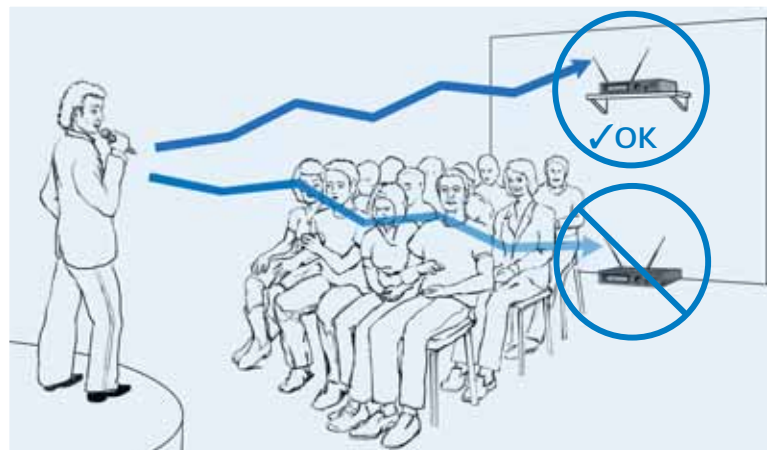
Figure 4-6: proper and improper antenna and receiver placement
